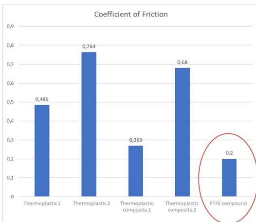
**Figure 3:** Comparison of coefficient of friction for different thermoplastics under dry friction conditions; counter surface stainless steel  $R_a \sim 0,3 \mu\text{m}$ ,  $R_z 2.5 \mu\text{m}$
